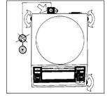
Afterwards, extend the auxiliary foot (22) until it touches the surface on which the balance is resting.
