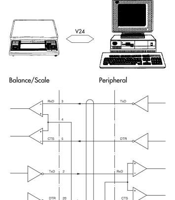
Type of cable: AWG 24 specification
