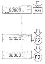
Press the tare key (10) for at least 2 seconds until "C-I" and "CAL" are displayed (next to the F1 key).
