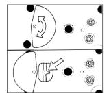
To fasten the hanger, open the below-balance port by turning the cover plate.
