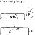
End of calibration: acoustic signal
