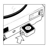
To fasten an antitheft locking device, use the lug (18) on the level indicator case of the balance.
