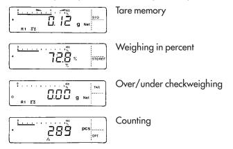
You can also use "tare memory" and "over/under checkweighing" in combination with "weighing in percent" or "counting."
