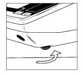
To level the balance using the level indicator as a guide:
