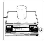
Center the calibration weight on the weighing pan.
