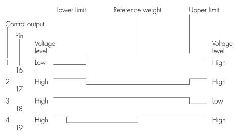
Control output 1: lighter Control output 2: equal Control output 3: heavier Control output 4: "set"
