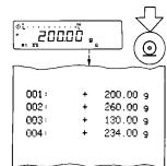
To print data on hard copy or have them output onscreen on an on-line computer, press the ② key (11).
