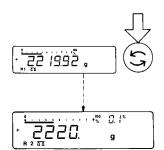
Oftentimes, a display accuracy of 2 grams is sufficient for a load of approx. 2 kg. In this case, it makes sense to select weighing range R 2 with an accuracy of 0.1% by pressing the Skey (8). While you are filling up to a target weight, it is certainly easier to work with a target of 2220 g than with an absolutely accurate readout of 2219.92 g.
