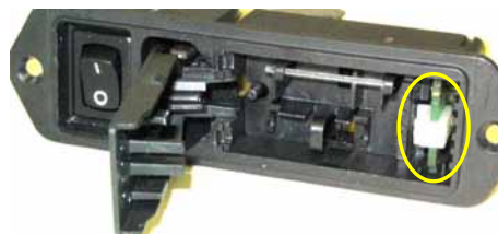
Fig. 5: Voltage selector board
