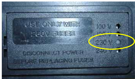
Fig. 3: Factory-set voltage selection, here: 230V
